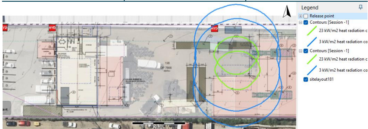
Figure 5-2: Radiant Heat Contours from Fire in Drop off (Incoming) Storage Area.
